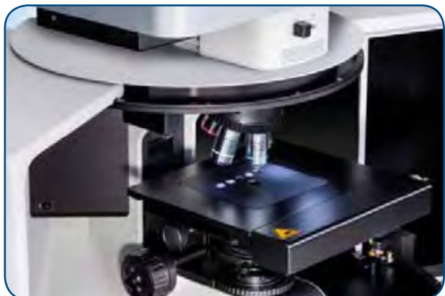
Validation plate with integrated standard materials for automated instrument qualification tests
