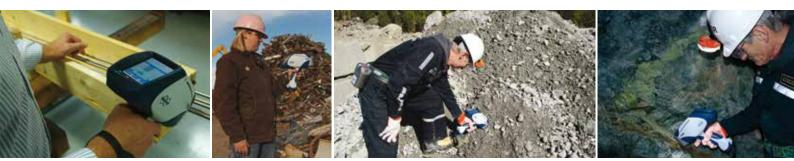
**Detector Technology:** With the introduction of the S1 TITAN model 500, Bruker becomes the first company to manufacture all industrial handheld XRF instruments using the latest Silicon Drift Detector (SDD) technology. This important step means that all instruments will have the latest in high resolution and high count rate detectors. As a result, the end user can expect to have fast, precise readings regardless of the model ordered.
