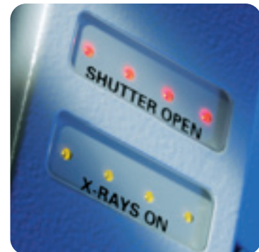
X-ray tube LED status display
