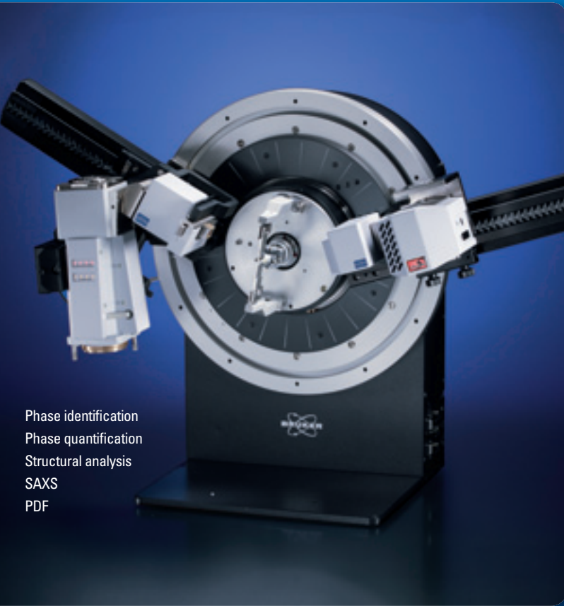
Capillary geometry with Johansson monochromator for pure K\alpha_1 radiation and LYNXEYE detector
