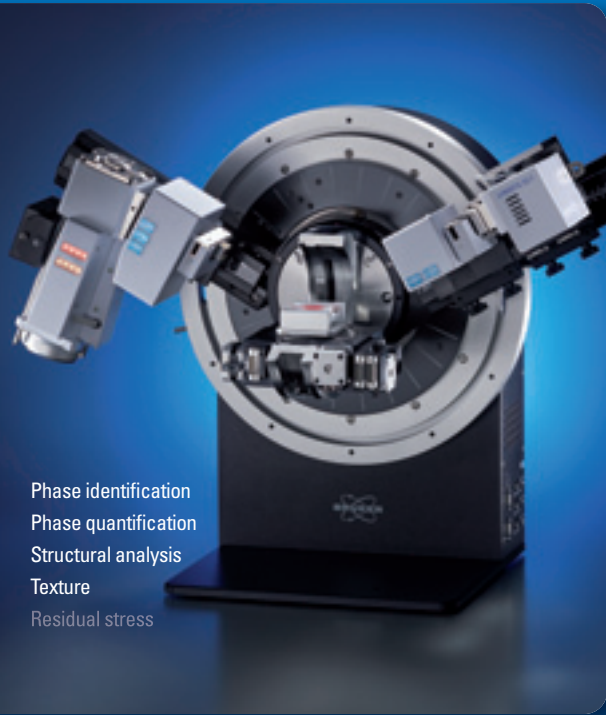
TRIO/TWIN setup in Bragg-Brentano geometry
