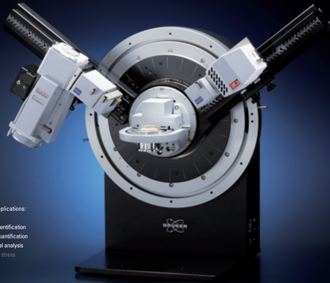
Bragg-Brentano geometry with LYNXEYE detector
