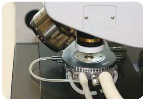
To investigate samples at certain temperatures from -196 – 600\text{ }^\circ\text{C} , the Linkam THM600 stage can be used. This stage is also controlled by OPUS software.
