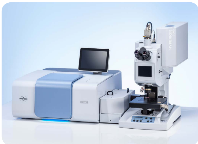
Figure 3: HYPERION 3000 FTIR imaging microscope coupled to an INVENIO spectrometer.
