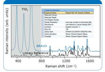
Figure 2: Identification of the composition of paint using the library SEARCH functionality of OPUS.
