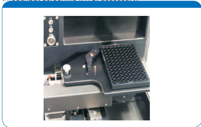
Fig. 4 HTS-Raman accessory mounted in the FT-Raman sample compartment
