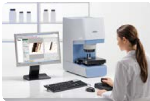
Analysis of small samples with the FTIR microscope LUMOS.
