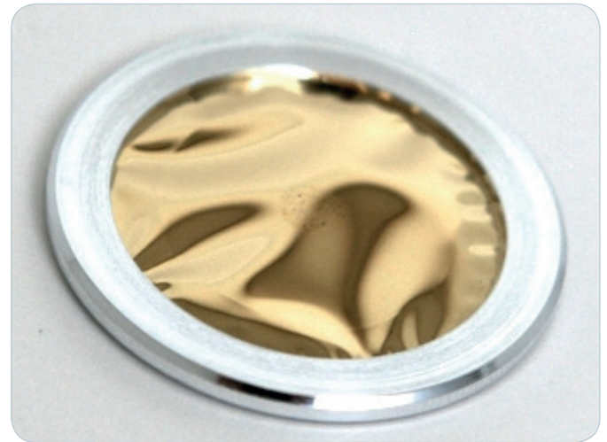
Fig 5: Gold filter for the isolation of particles from liquid formulations
