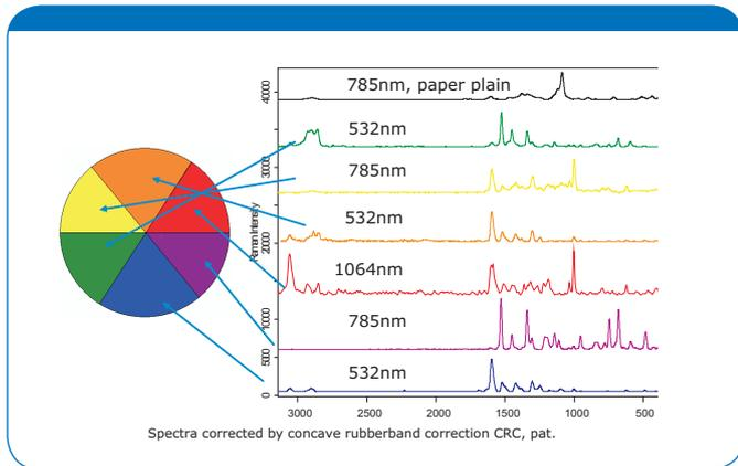
**Fig. 6** RamanScopell In Situ Analysis of Laserjet Ink
