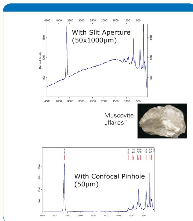
Fig. 1 Removing Fluorescence by Confocal Raman Microscopy
