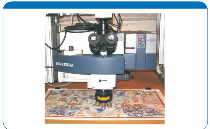
**Fig. 7** Open-Architecture Raman Microscope
