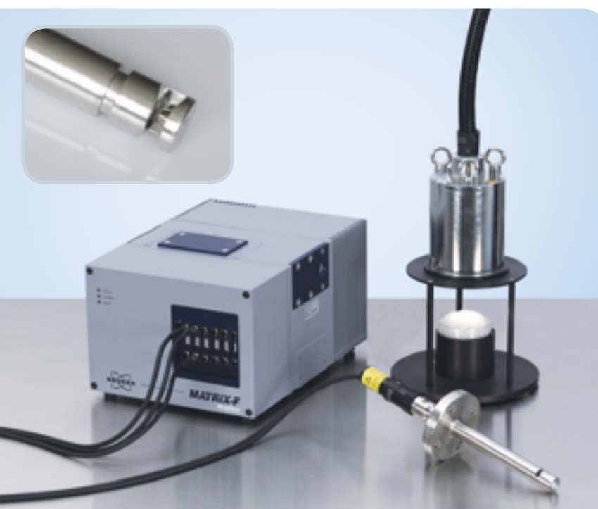
MATRIX-F FT-NIR spectrometer for the on-line control of liquid and solid products
