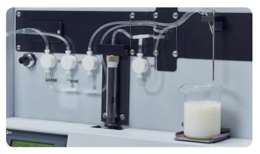
The GLOBULYSER measures the homogenizer efficinecy for various types of milk and liquid milk products.
