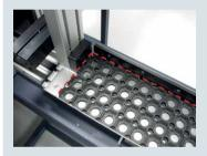
Robust mechanical stops (here: for square ingots) and a precise linear stage ensure the X-positioning accuracy of the ingot. For all SBS versions (square or cylindrical ingots) the support area is realized such that slipping or rolling of the ingot during the measurement is not possible.
