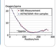
SBS results correlate perfectly with quantification according to ASTM/SEMI 1188, proving the accuracy of SBS analysis.
