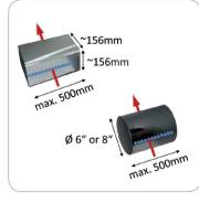
Three different SBS versions are available for square standard PV ingots or for cylindrical ingots with either 6" or 8" diameter.
