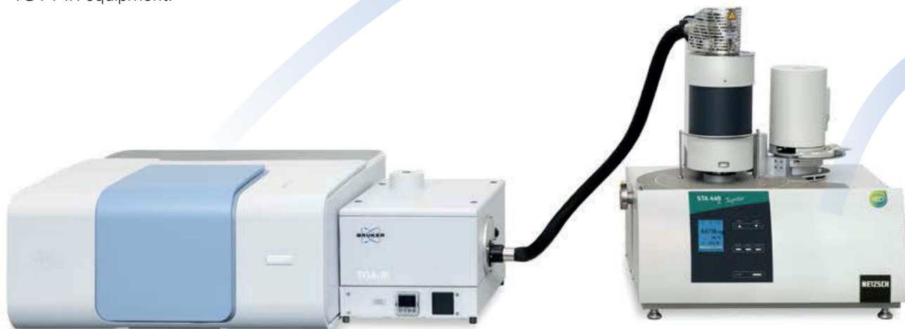
Bruker INVENIO with external gas cell
