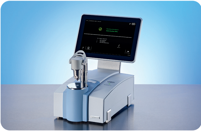
Figure 1: ALPHA II FTIR spectrometer with touch panel PC and Platinum ATR-module
