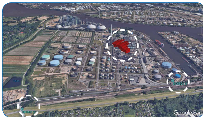
Figure 4: 3-D identification model of a gas cloud above an industrial emission stack displayed in Google Earth™.
