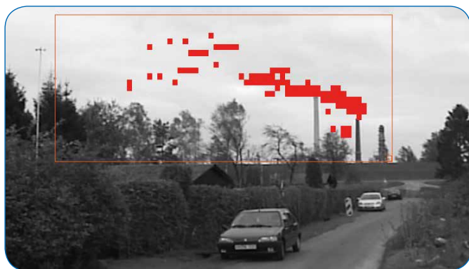
Figure 3: 2-D identification image of a gas cloud above an industrial emission stack of a refinery measured by the SIGIS 2.
