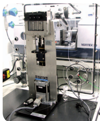
Photo showing stopped flow unit in foreground and VERTEX 80 with IR cell in background
