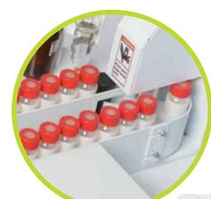
**Sample Conveyor** – The Lotix conveyor systematically moves sample vials to and from the sample position for sample introduction via the needle assembly. The conveyor is designed to hold 30 – 40 mL VOA vials.
