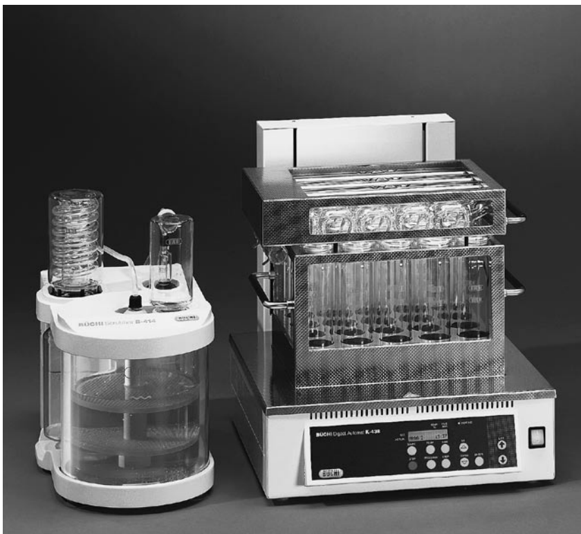
Figure 5: Scrubber B-414 connected to a Digestion Unit K-438.
