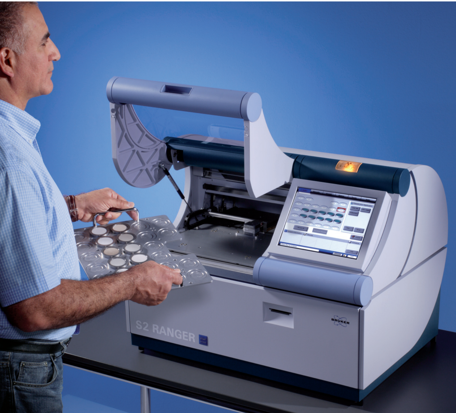
S2 RANGER with sample changer and tray for 28 samples
