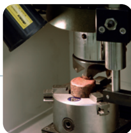
■ Check sample height at molding cutter
