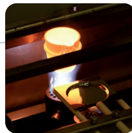
■ Heat crucible in melting furnace
