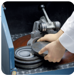
■ Mill in grinding vessel
