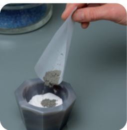
■ Add sample to flux material
