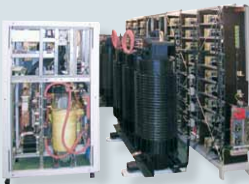
Klystron power supply for the MAMI C race track microtron, Mainz University, Germany.
