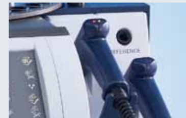
Fiber Optic Probes for measuring samples directly in sample containers.
