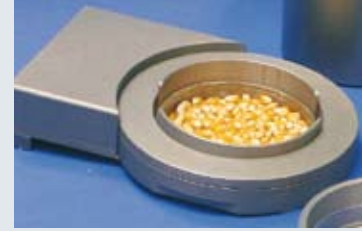
Optional rotating cups in different sizes can be mounted off-centered on the sample window of the MATRIX-I for averaging sample inhomogeneity.
