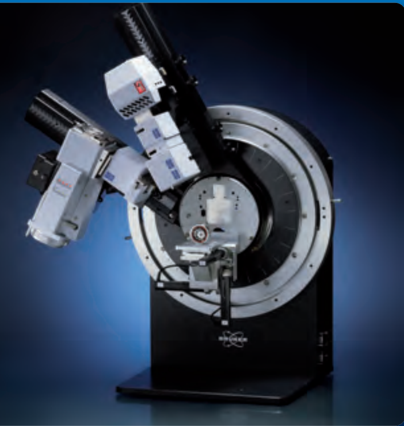
Stress measurements in iso-inclination (omega) mode
