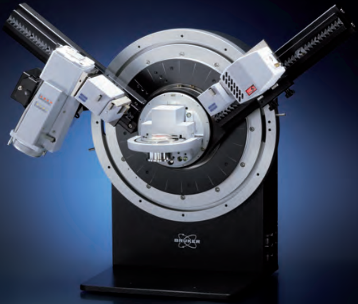
Bragg-Brentano geometry with LYNXEYE detector
