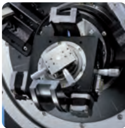
Compact Eulerian cradle with XY stage
