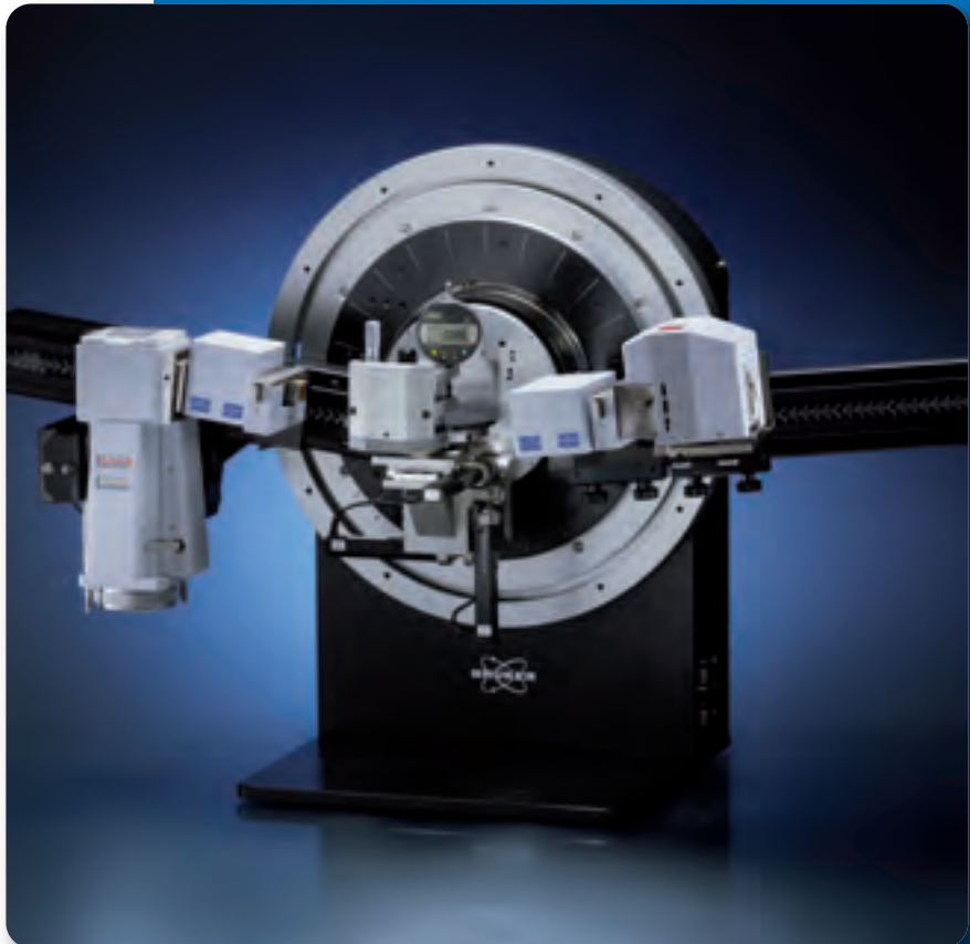
Reflectometry TWIN/TWIN setup with LYNXEYE detector in 90° position
