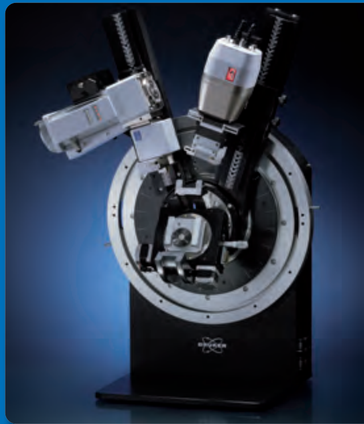
Texture or stress measurements in side-inclination (psi) mode
