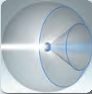
Uniform diffraction signal along Debye rings
